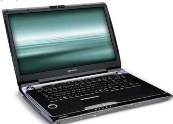
Figure 2 – The Toshiba Qosmio G55 Series includes a DSP like ‘Cell’ processor to give a 10-fold speed boost for video encoding tasks and enable features such as facial and gesture recognition.
